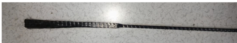
Fig. 6. The scattered end of the CFRP cable [99].
